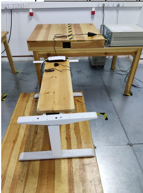
Test setup: EFT & Voltage Dips & Surge
