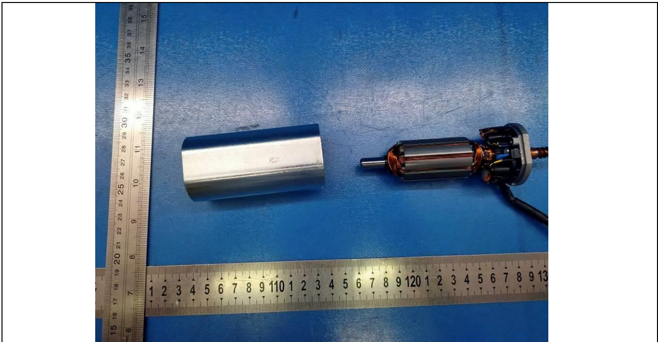
Details of: Internal view of Motor(3045D024)
